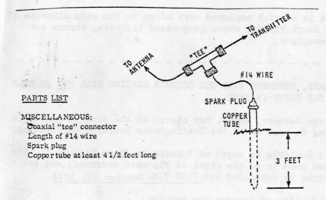
The drawing on the cover is an inexpensive Lightning Arrester. The whole thing consists of a junkbox collection of components: a coax "tee" connector, a few coax connectors, a spark plug, a short length of #14 manget wire, and some copper tubing. A spot near the ground is selected on the feedline and the coax is clipped. The coax connectors are then affixed to each end of the cut feedline. The "tee" connector is now inserted between these couplings.
